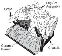
Figure 1 - Product Identification (Ramp Pan Burner)
